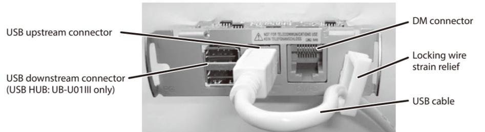
3. Insert the square connector end of the USB cable into the upstream connector of the UB-Board.
