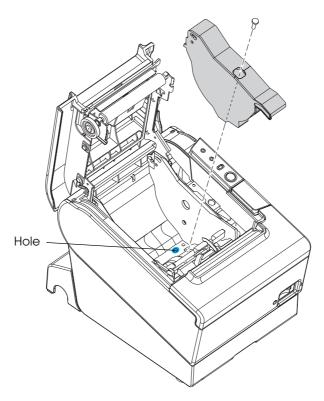
3 Tighten the enclosed screw to fix the roll paper guide.
