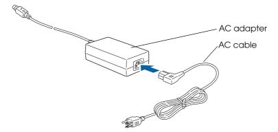
3 Insert the connector of the power supply cable onto the power supply connector (stamped **24V**).
