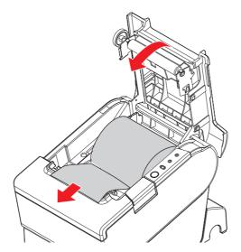
5 Tear off the roll paper with the manual cutter.
