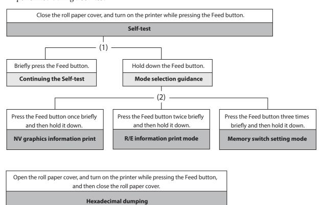
In (1) and (2), the following guidances are printed, the Power LED flashes, and instructs the user's operations.
