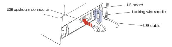
3 Connect the USB cable from the host computer to the USB upstream connector.
