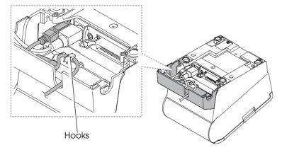
After the cable arrangement, turn over the printer, and make sure the cables are not pinched.
