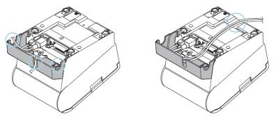
If you want to pass the USB cable through the cable exit on the back, fit the cable under the hook on the printer to prevent the cable from coming off.
