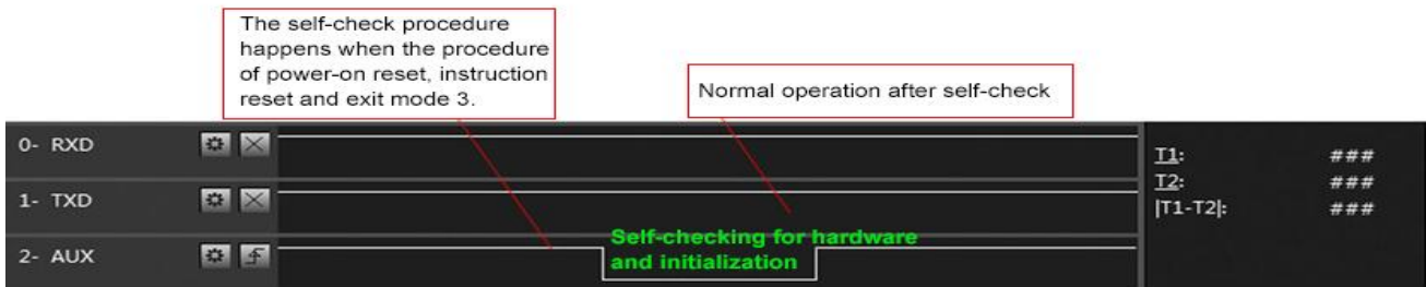
Timing Sequence Diagram of AUX when self-check
