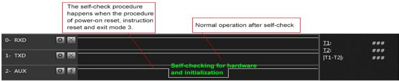
Timing Sequence Diagram of AUX when self-check
